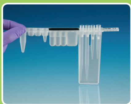
Add user-defined primers/probes to unitized reagent strips – load rack(s)
